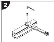
Arm is fitted in pinion with hex head screws.
