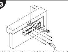
Using the templates provided, fix the mechanism to the door as well as the armset and any necessary brackets.
