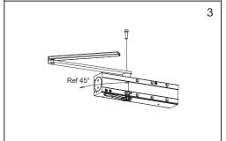
Rotate the bottom pinion to approximately 45° with a wrench as illustrated and then assemble the main arm.
